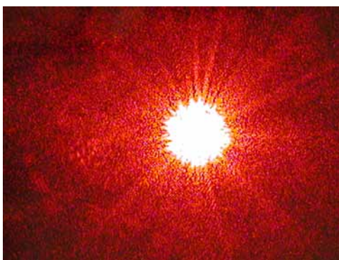
A beam of light is refracted through a glass slide sprayed with Surround.
